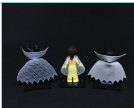
Fig. 13: Multi-material gripper (ABS, TPU 33 Shore D)
