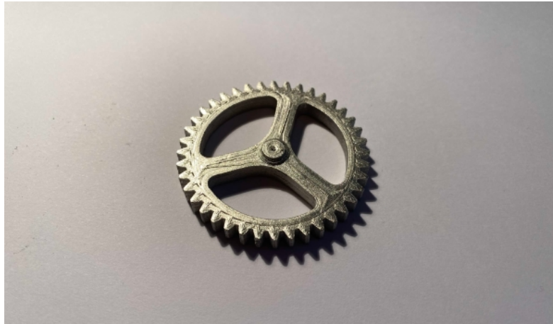
Sprocket in 17-4 PH stainless steel printed on a PAM 3D printer in sintered state.
