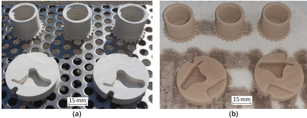
Figure 8 - Parts after the two stages of debinding: (a) 1st stage by aqueous debinding; (b) 2nd stage by thermal debinding.
