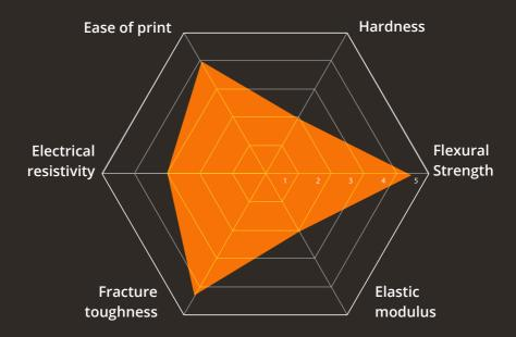
Zirconia or Zirconium oxide is a chemical compound of Zircon and oxygen with the chemical formula  $ZrO_2$ . With no pigment, it is an ivory colored ceramic. Zirconia is a multi-purpose construction material with a very low thermal conductivity and high strength. Components made from this material are significantly more expensive than components made of alumina ceramics.
