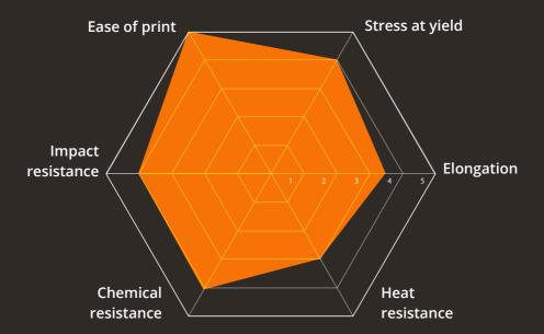
TPU Natural is a flexible thermoplastic that can print many parts that require great flexibility. This material presents high wear and abrasion resistance, high tensile strength and resistance to tear propagation, good damping characteristics and offers a high resistance to chemical. It is ideally suited for industrial applications and offers a high quality of resolution when printed.
