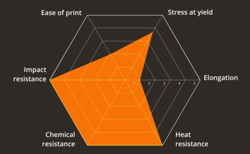
PPS is a semi-cristalline high performances thermoplastic with excellent mechanical and chemical resistance.
