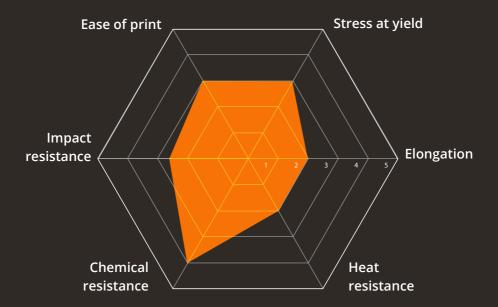
PP is a polyolefin semi-cristalline polymer and its properties are closely linked to its morphology and molecular structure. Lightweight, stiff at high temperature and chemically stable it is a commodity thermoplastic which is most often preferred to PEBD. Glass fiber or other fillings can be used to increase stiffness.
