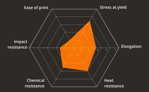
POM is an engineering thermoplastic mainly used in replacing metallic solution where high stiffness, low friction and good dimensional stability are required over a large temperature range. POM can be impact resistance modified or glass fiber reinforced to reach higher stiffness at elevated temperature.
