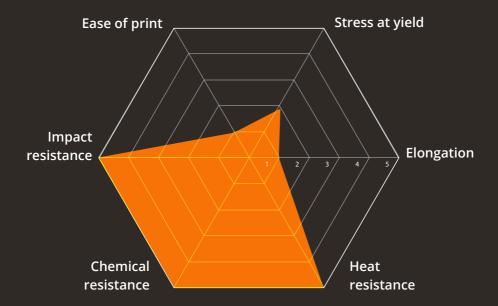
PESU is a high-performance materials with a temperature profile that is unique among engineering thermoplastics a long-term temperature resistance up to 180°C. It is used in sectors as a substitute for glass, metal, ceramic, and porcelain.
