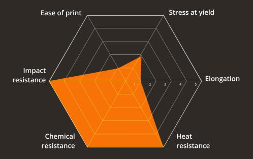
PEEK is a semi-cristalline high performance thermoplastic with excellent mechanical, chemical and impact resistance properties over a large range of temperature, which make PEEK and its derivatives a unique class of thermoplastic. The high purity of the molecular structure makes PEEK sterilizable and biocompatible. PEEK can be reinforced with glass or carbone fiber to reach severe application requirements.
