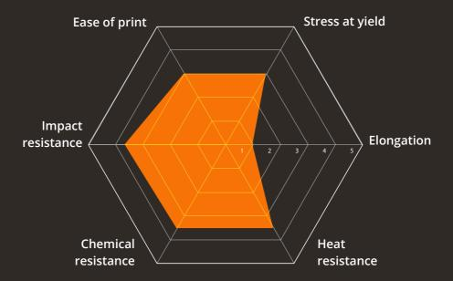
PC is an amorphous engineering thermoplastic with high mechanical properties, good heat resistance and excellent transparency. PC can be glass fiber reinforced and impact resistance modified.
