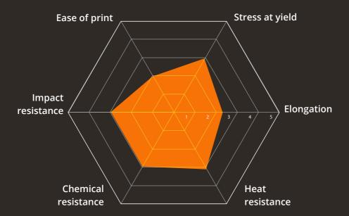
Polyamide 6 also called polycaprolactam, is a semi-crystalline thermoplastic. PA6 is used for the production of technical parts requiring good mechanical resistance. It has a low coefficient of friction, good thermal resistance and electrical insulation properties.
