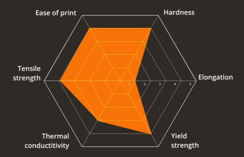
M2 steel is the "standard" and most widely used industrial Highspeed steel, commonly used as cutting tool material. It is often used in power-saw blades and drill bits. After heat treatment, its hardness is the same as T1, but its toughness and thermo-plasticity are higher than T1 by 50%.
