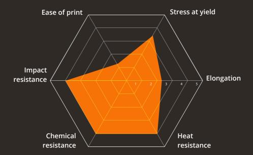
HPP offers strength and durability that provides an outstanding combination of mechanical properties and toughness. Chemical resistance and hydrolytic stability are improved compare to other copolyesters.
