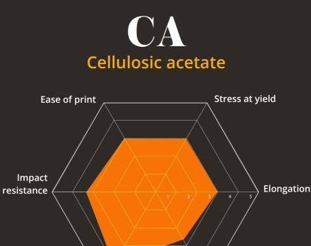
Cellulosic acetate material are esters bio-based polymers. They are produced through reaction of cellulose with organic acids, anhydrides or acid chlorides. Cellulose acetate is one of the oldest bio-based polymers in the world. Due to its properties, thermoplastic CA is a promising biopolymer for replacing PS in certain foam applications.
