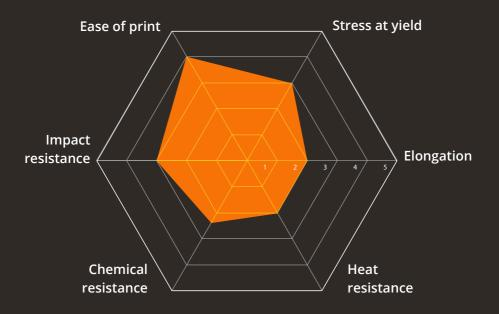
ASA is an amorphous styrenic copolymer, it is structurally very similar to ABS. It presents high surface quality, good impact strength, chemical, UV and heat resistance. For these reasons, ASA is used as the material of choice for exterior applications. This material can be easier to 3D print than ABS.
