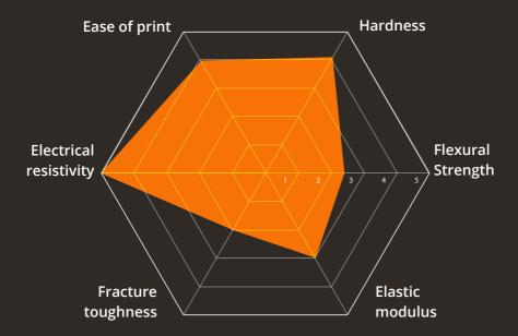
Alumina or aluminum oxide is a chemical compound of aluminium and oxygen with the chemical formula  $Al_2O_3$ . Is the most well-known oxide ceramic material. Aluminum oxide is an electrical insulator and has a relatively high thermal conductivity (30  $Wm^{-1}K^{-1}$ ). Due to its relatively high hardness, it is used as an abrasive and a component in cutting tools.
