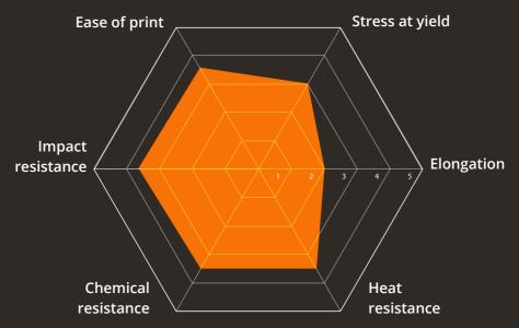
ABS/PC blend combines the properties of PC and ABS, in other words the high processing capacity of ABS with excellent mechanical properties, resistance to heat and impact, from the PC. The level of the two components affects the heat resistance.
