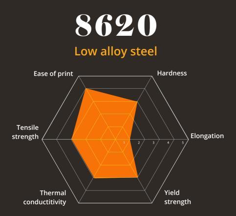
8620 steel is a low alloy steel. It is a common, case hardenable (carburizing) alloy. It is a responsive to mechanical and heat treatments than carbon steels. It is utilized for various applications requiring good tensile strength and reasonable toughness.
