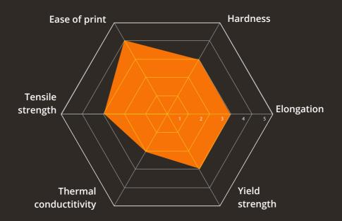
304L stainless steel is the most common stainless steel, as 316L stainless steel it is non-magnetic, austenitic, corrosion resistant alloy. With its low carbon content, 304L steel minimizes the risk of precipitation of chromium carbide and therefore offers better protection against corrosion.
